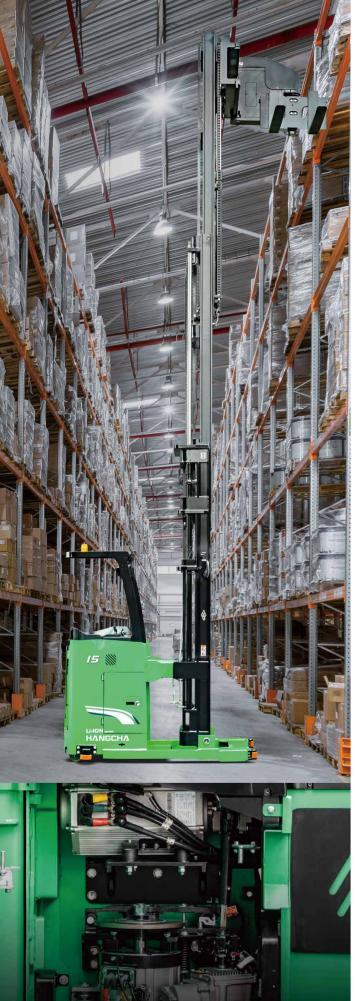
The oil pump motor assembly is provided on the rear side of the stacker, so that the center of gravity of the whole stacker moves backwards and the stability is better.
